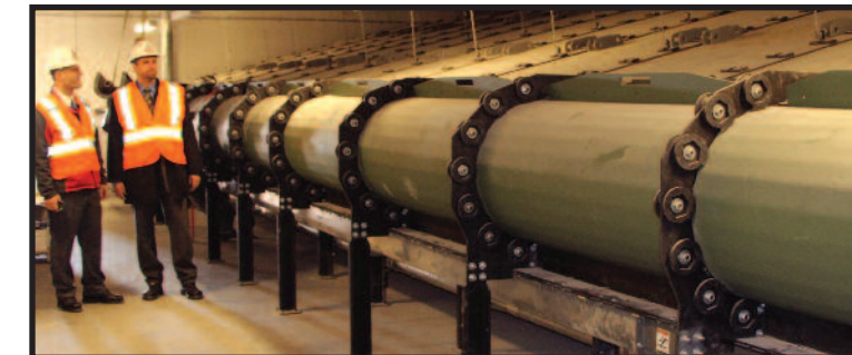
Deputy Chief Paul Martin and CAO Stan MacLellan inspect the bullet trap at the new OTC shooting range.
